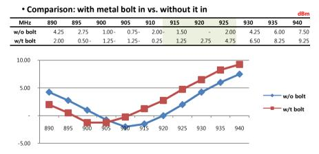
•BASIC reads best without any metal bolt in two holes (located diagonal directions). With RF interference, metal bolts decreases read range by 30% or more. RFcamp recommends not using metal bolts, but 3M 300LSE adhesive or glue for maintaining optimum read performance. In case adhesive or glue can not be used, polycarbonate (or nylon) bolts is recommended.
