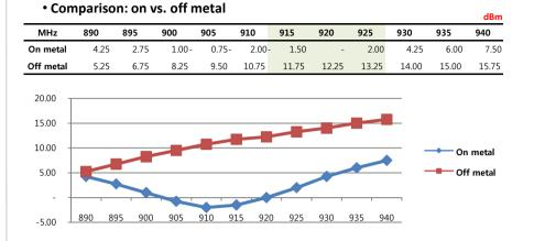
•BASIC reads shorter by 70% or less off metal (or on non metal surface). It can be applied, therefore, only for metal application. For non metal application, please use PALLET.
